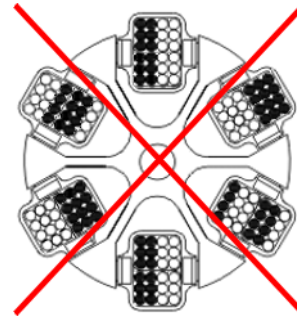
Fig. 20: Permissible and impermissible loading of an angle rotor and a swing-out rotor (example illustration)
