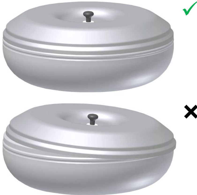
Fig. 18: Checking the cover for correct fit
