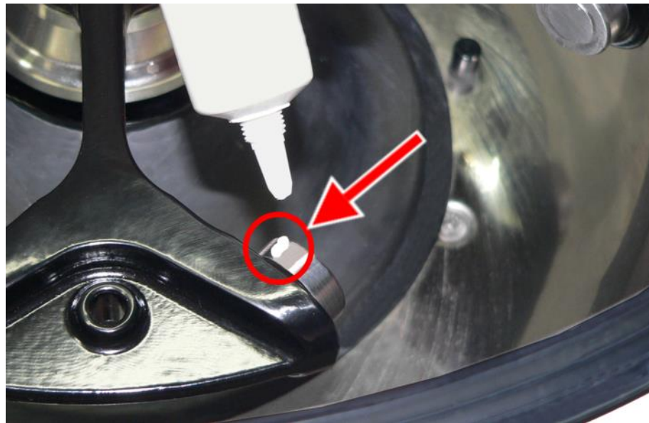
Fig. 46: Sufficient quantity of grease for one bolt
