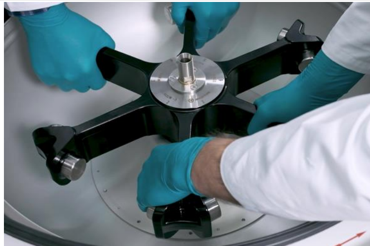
Fig. 16: Correct method for lifting the rotor 11805
