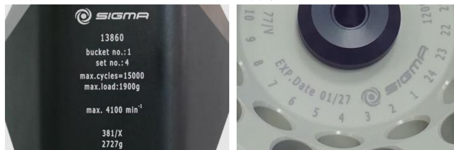
Fig. 8: Different service life – engraving on the bucket/rotor
