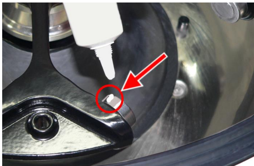
Fig. 38: Sufficient quantity of grease for one bolt
