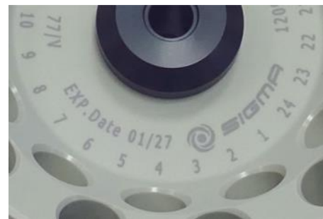
Fig. 6: Different service life – engraving on the bucket/rotor
