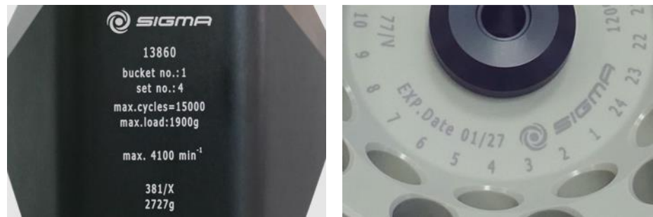
Fig. 5: Different service life – engraving on the bucket/rotor
