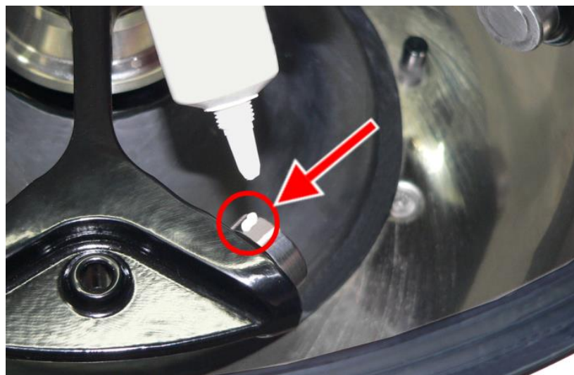
Fig. 37: Sufficient quantity of grease for one bolt
