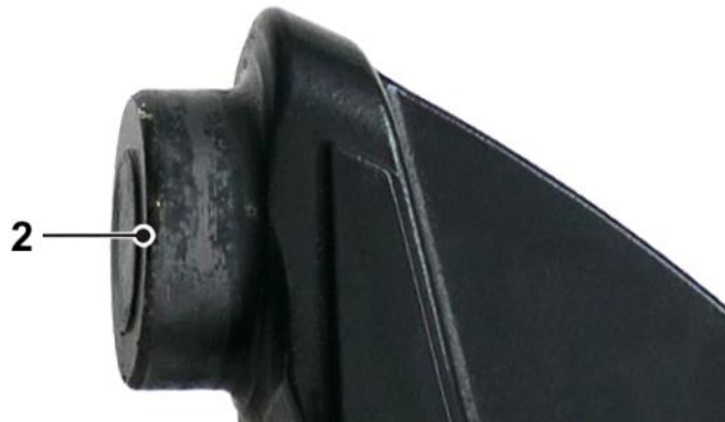
Fig. 8: Load-bearing bolt with traces of use – no greasing required
