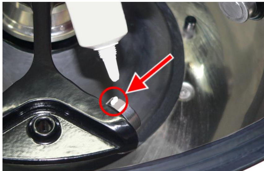
Fig. 37: Sufficient quantity of grease for one bolt
