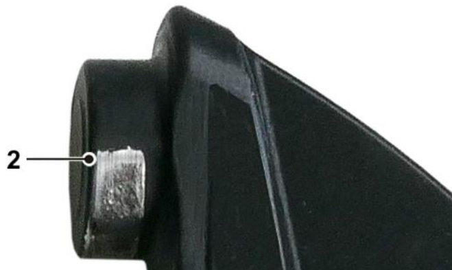
Fig. 9: Load-bearing bolt with completely worn-off anti-friction coating – greasing required
