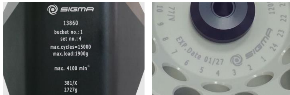
Fig. 5: Different service life – engraving on the bucket/rotor
