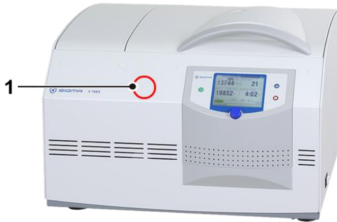
Fig. 35: Position of the opening for the emergency lid release
