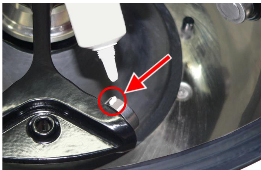
Fig. 38: Sufficient quantity of grease for one bolt
