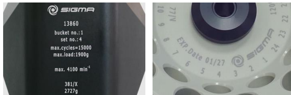
Fig. 7: Different service life – engraving on the bucket/rotor
