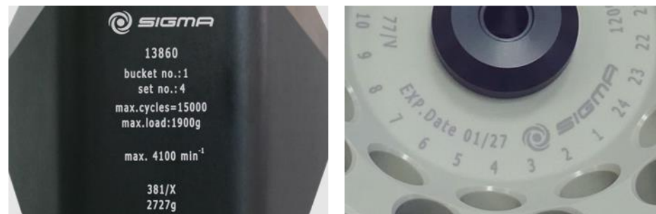
Fig. 5: Different service life – engraving on the bucket/rotor
