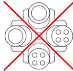
Fig. 11: Permissible and impermissible loading of a swing-out rotor with vessels of various sizes (example illustration)
