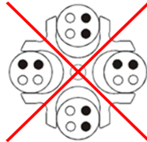
Fig. 12: Permissible and impermissible loading of an angle rotor and a swing-out rotor (example illustrations)
