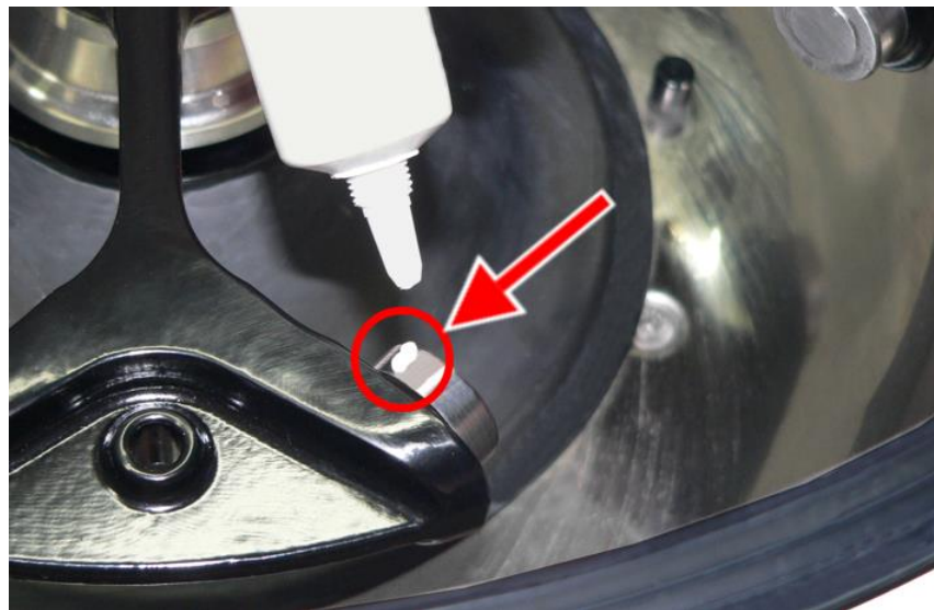
Fig. 35: Sufficient quantity of grease for one bolt
