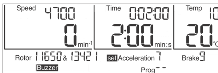
Fig. 23: Preselection of a curve; here: preselection of an acceleration curve
