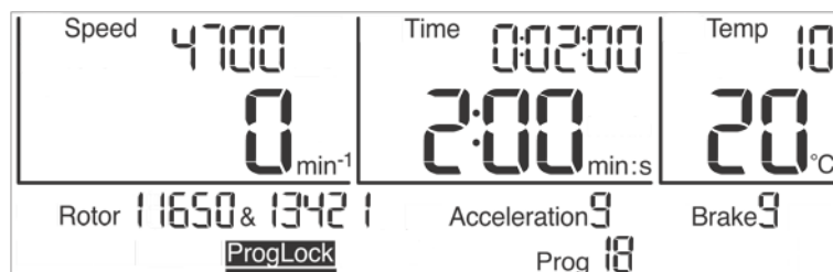
Fig. 26: The program lock "ProgLock" is activated
