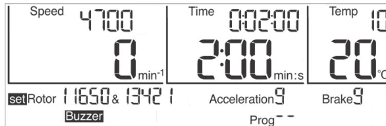
Fig. 22: Preselection of a rotor or a rotor/bucket combination
