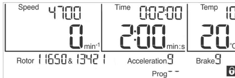
Fig. 29: "Padlock" symbol indicating an activated input lock
