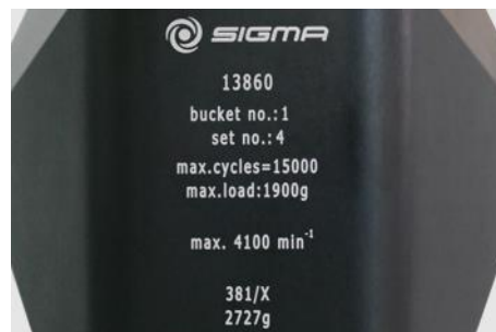
Fig. 5: Different service life – engraving on the bucket/rotor
