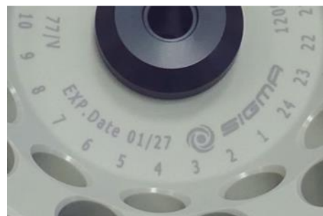
Fig. 5: Different service life – engraving on the bucket/rotor
