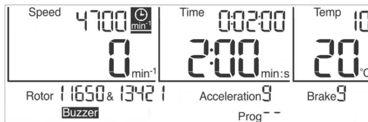
Fig. 17: The function "Runtime as of the set speed" is activated
