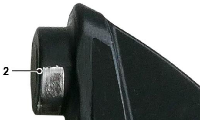
Fig. 8: Load-bearing bolt with completely worn-off anti-friction coating – greasing required
