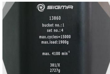
Fig. 4: Different service life – engraving on the bucket/rotor
