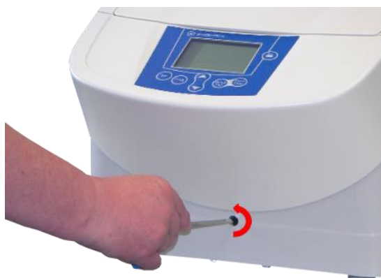
Fig. 11: Manual release of the lid lock
