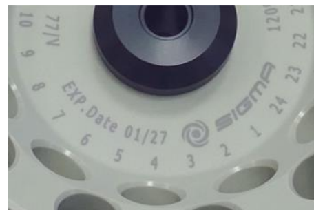
Fig. 4: Different service life – engraving on the bucket/rotor
