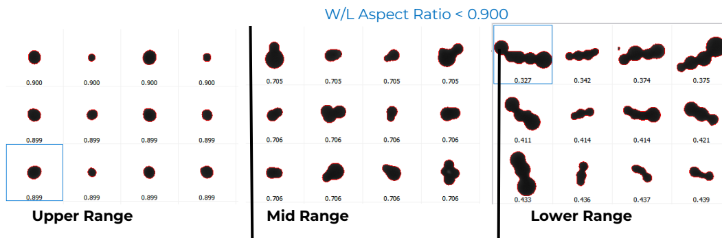
Figure 14. Selected images in W/L range less than 0.900. As W/L decreases, images show increasingly fused individual powder particles. QC departments can use images as guides for setting their specifications on shapes.
